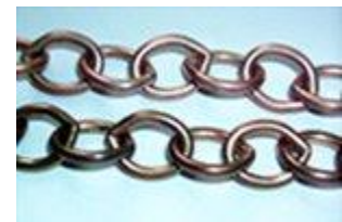
Top: Brass chain cleaned with vinegar and salt solution. Bottom: Tarnished chain.
