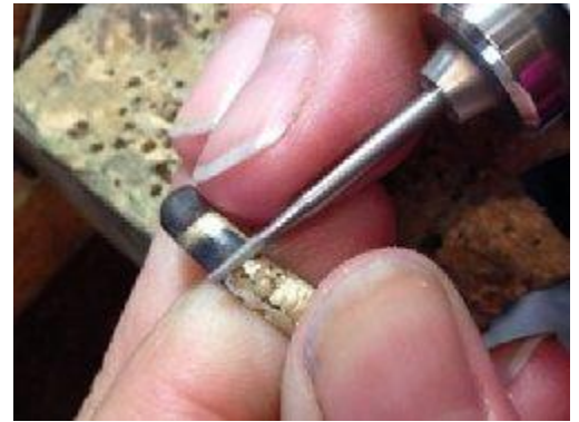
Masterful Kate removes visible solder with a tapered barrel bur in a flex shaft.
